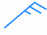
Figure 7: Wind glyph used in the Skew-T. This specific glyph is showing a wind from 045° at 25 knots.
