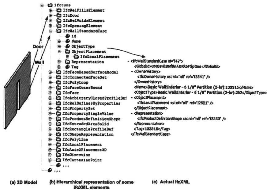
Figure 1: Structure of ifcXML data.
