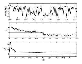
Figure 2: The top plot shows the one-step-ahead output predictions [--] and the true outputs  $[\cdots]$  for the RBF model. The middle and bottom plots show the true values and estimates of the model order and noise variance respectively.
