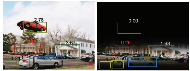
Figure 8: An object which is out of context may be falsely eliminated by our system.
