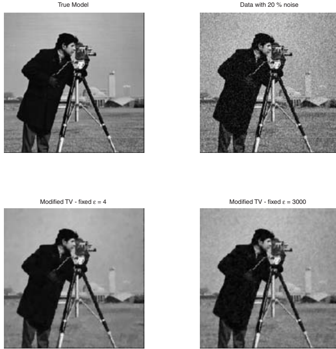
FIG. 1. Denoising: The “true image” (upper left) is corrupted by adding 20% white noise (upper right) and the latter is fed as data b to a denoising program using the usual Tikhonov regularization with modified TV. The smaller value of switching parameter \varepsilon (lower left) produces a more pleasing result than the larger value (lower right). Taking \varepsilon = .01 or \varepsilon = 10^{-6} yields results similar to those displayed in the lower left panel but at a higher cost.
