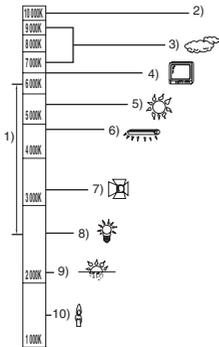
Outside of the effective range of automatic white balance adjustment, the image will become reddish or bluish. Even within the effective range of automatic white balance adjustment, the automatic white balance adjustment may not function properly if there is more than one light source. For light outside the functional auto white balance adjustment range, use the manual white balance adjustment mode.
