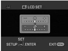
2 Move the joystick up or down in order to select the item to be adjusted.
