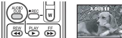
**4** Press the [II] button on the remote control to start audio dubbing.
